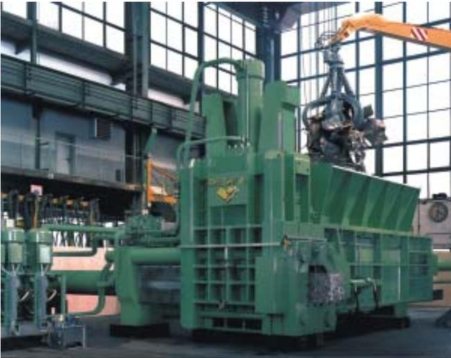
Producing a great deal of noise, unshapely pieces of sheet metal punched out during production fall down to the lower storeys into the meter-long filler channel of the hydraulic press, where an initial hydraulic cylinder pushes them several meters into the pressing chamber. Here, the cylinders press the shapeless pieces of metal into a space-saving block, which is then transported away for recycling.
