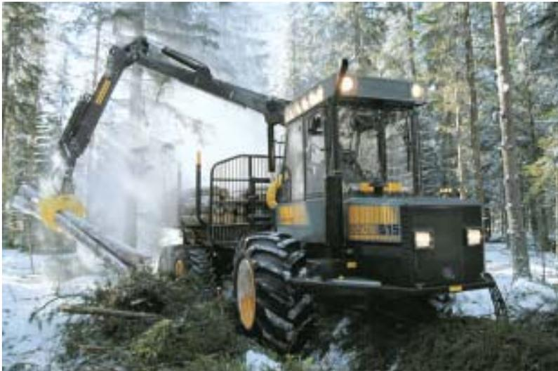
For the transport of the timber to paved roadways forwarders are used which can transport up to 14 tonnes of material. These are equipped with a telescopic crane which can grip tree trunks from a distance of 10 m.
