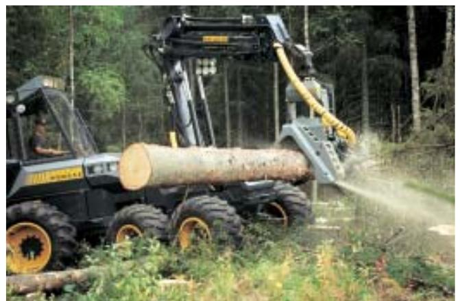
The harvester fells, measures, disbranches and cuts the trees into lengths within a few seconds for further processing of the trunks.
